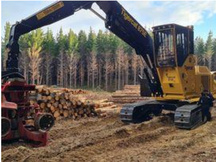
Our new Tigercat 87E harvester with a Waratah HTH624C Processing Head.
